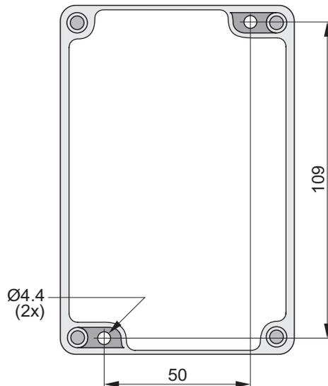
**Fig. 3.1: fixing holes**
