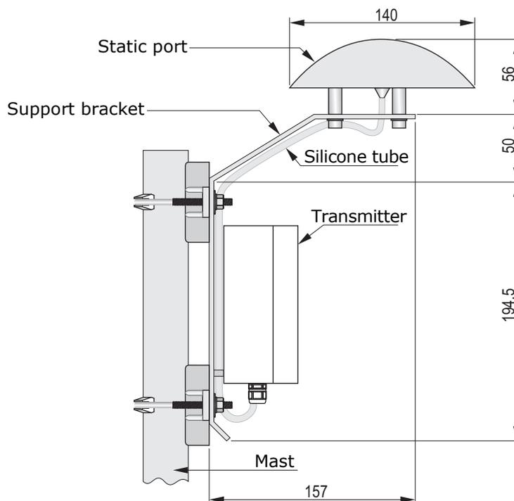
**Fig. 3.2: transmitter with static pressure port**
