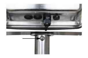
Use the screw of the adapter to fix the display unit on the tripod.
