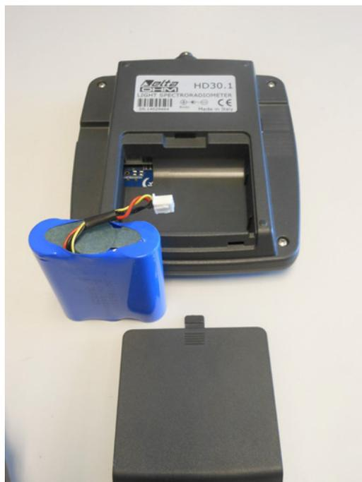
*Figure 2.2: Battery removed from housing.*
