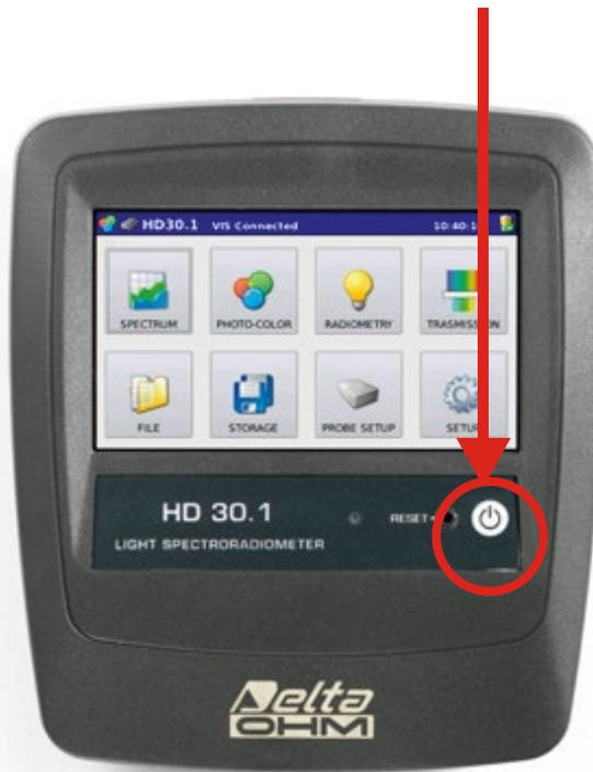
Fig. 6.4 : Monitor reactivation button
