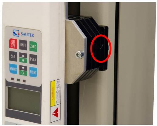
1.4 Now you can mount the clamp to the force gauge (here AE 500, red marking)
