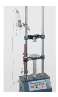
• The force gauge screwed to the test stand is now connected to the test stand at the equipment port by means of the RS232 cable
