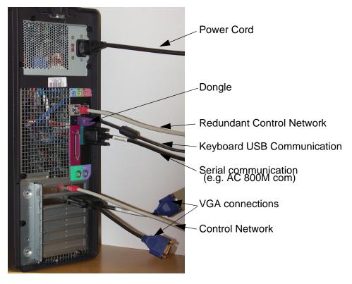
Figure 5. Rear side PC connections
