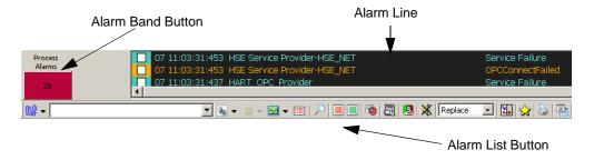
Figure 64. Accessing the Process Alarm List
