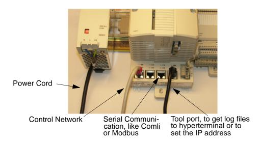
Figure 20. AC 800M connections
