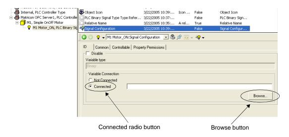
Figure 28. Connect the Signals
