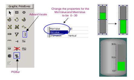
Figure 113. Bar Graph added to Tank Element
