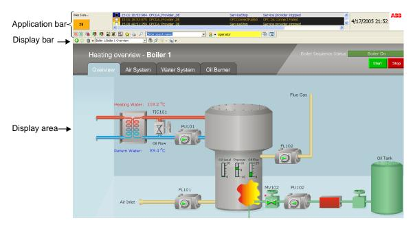
Figure 53. Operator Workplace in Operator Mode
