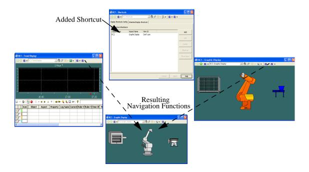
By adding a shortcut to the RC1 object, pointing to the RC2 Graphic Display, the RC2 Graphic Display can be accessed both from the RC1 Graphics Display and the RC1 Trend Display.
