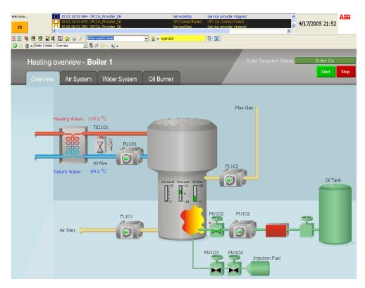
Figure 3. The Operator Workplace Window
