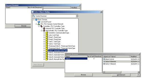
Figure 126. Inserting PLC Connect Element in Graphic Display
