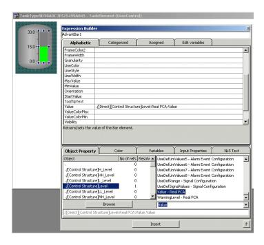
Figure 114. Connecting the Bar Graph
