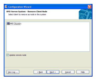
Figure 87. Remove a Client Node
