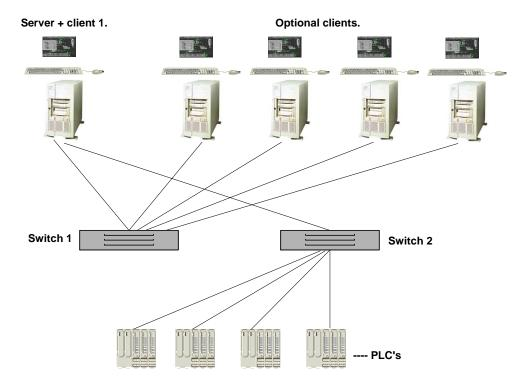
Figure 7. Separate Network Setup
