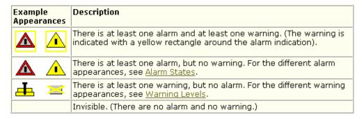
Figure 104. AlarmWarning Combo Appearance
