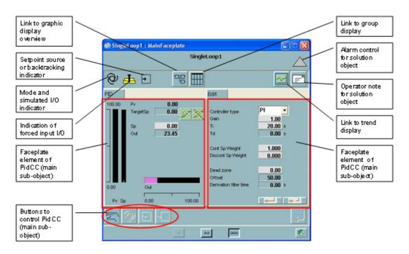
Figure 106. Extended faceplate of SingleLoop solution
