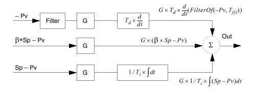
Figure 36. The principle of an ideal PID controller
