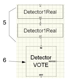
Figure 229. Two Smoke detectors and a connected Vote module presented in the CMD Editor for FireAreaFA11
