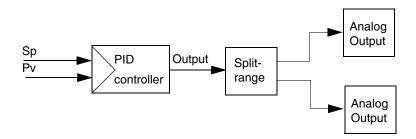
Figure 56. Example of split-range control where the output range from the controller is divided into two branches with different ranges
