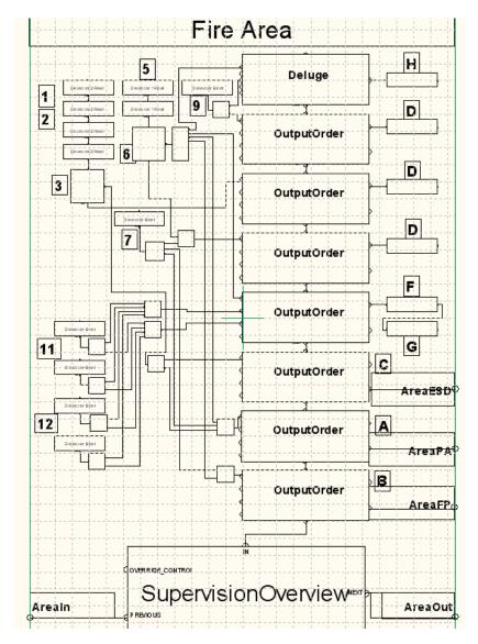
Figure 219. The FireAreaFA11 in the CMD Editor, with letters and numbers corresponding to the fire protection data sheet
