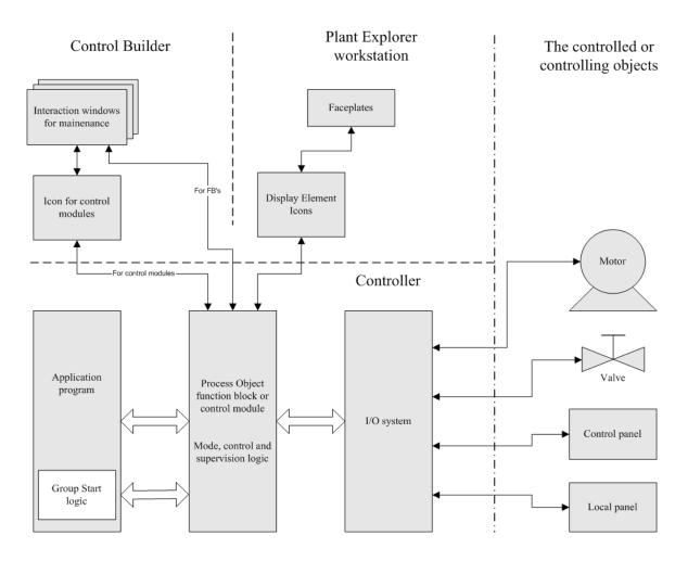
Figure 150. Relations between a function block or control module and the remote objects
