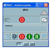
Figure 163. Example of reduced faceplate (BiM)
