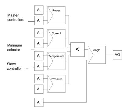
Figure 138. Example using control modules for override control in a heat pump using a minimum selector control module
