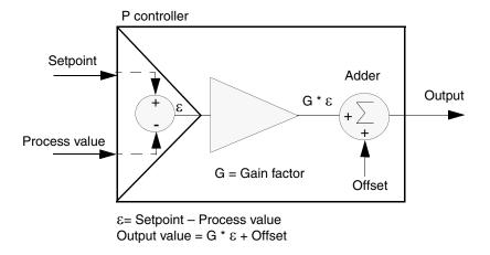
Figure 35. The basic P controller
