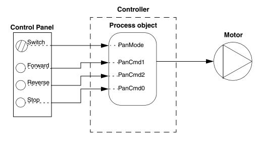
Figure 189. The Panel mode control diagram. A general solution for smaller applications, where all four Panel parameters are connected from a control panel
