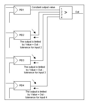
Figure 137. Example of a Max4CC control module with inputs from controller outputs
