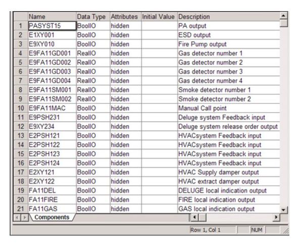
Figure 218. The components inside the IO\_connections data type
