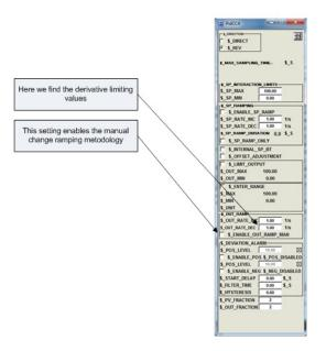
Figure 41. The interaction window of a PidCC or PidAdvancedCC
