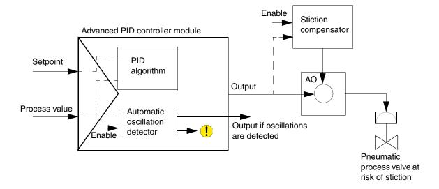
Figure 95. Principles for detecting and solving friction problems
