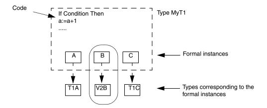
Figure 25. Copy of template type with formal instances, modified by replacing one of the formal instances (circled in the figure)
