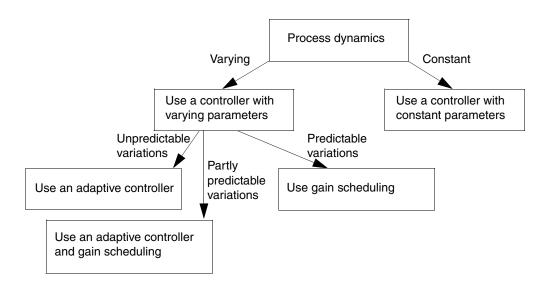
Figure 93. Procedure used to decide which controller to use, adaptive control and/or gain scheduling
