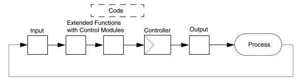
Figure 51. A control loop with all functions defined by control modules from the control libraries
