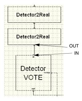
Figure 226. The Detector Vote module graphically connected to the last Detector2Real gas module
