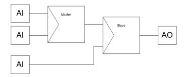
Figure 136. Example of a cascade control loop consisting of control modules
