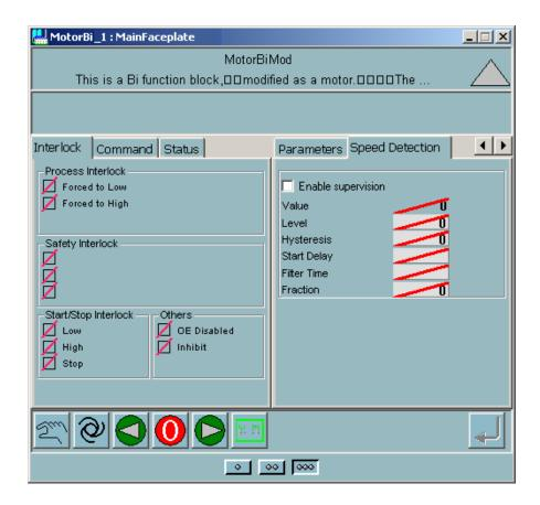
Figure 256. The newly added Speed Detection tab in the extended faceplate
