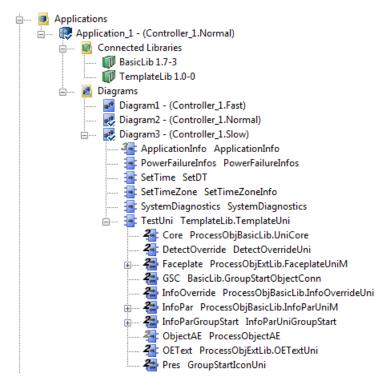
Figure 19. TemplateUni used in a diagram under the application
