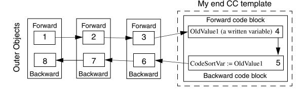
Figure 60. My end CC template object has an end solution. It stops passing information forward and begins passing information backwards to the next backward block
