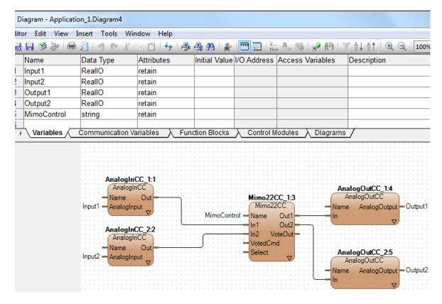
Figure 79. Mimo22CC connected in diagram editor
