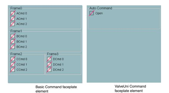
Figure 173. The basic Command faceplate element and the corresponding one in the ValveUni(M) type
