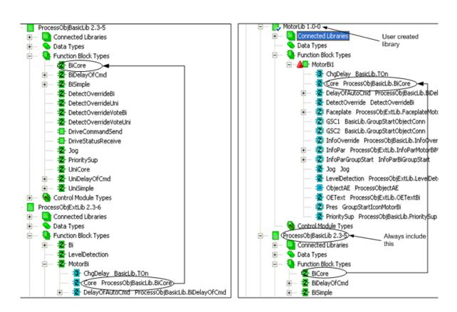
Figure 151. The core functionality in ProcessObjExtLib and in a user's self-defined library
