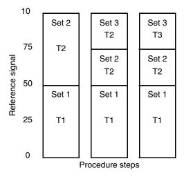
Figure 92. Example of the procedure for gain scheduling in three sets
