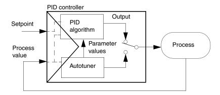
Figure 86. The principle of autotuning in a PID controller with the Autotuner function
