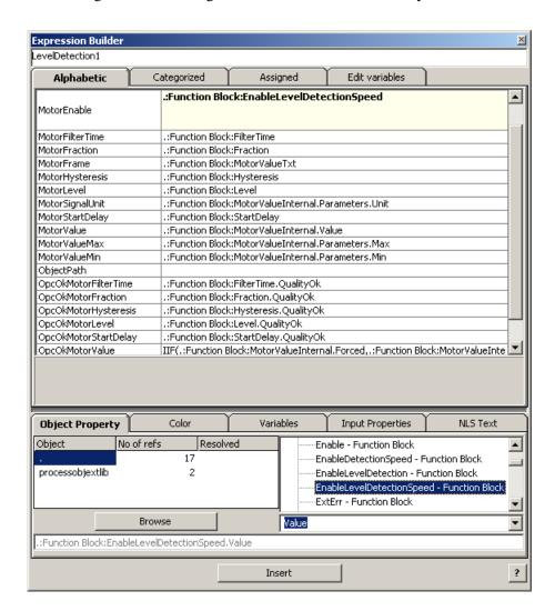
Figure 181. Changing the signals from EnableLevelDetection to EnableLevelDetectionSpeed in the Expression Builder window
