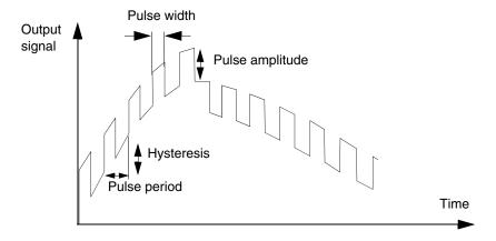
Figure 97. The stiction compensator signal is superimposed on the analog output signal
