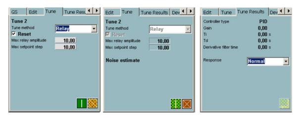
Figure 48. Autotuning in a PidAdvancedCC control module
