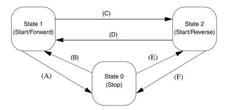
Figure 158. Manual maneuvers interlocking signals
