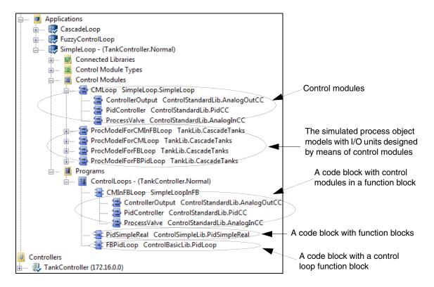
Figure 144. The four methods of designing an application and the simulated process
