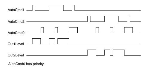
Figure 156. Status relations of OutLevel parameters and Auto commands (BiCore)
