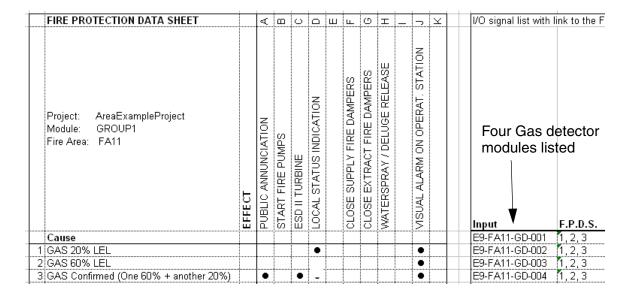
Figure 220. Part of the data sheet presenting information for Gas detection
