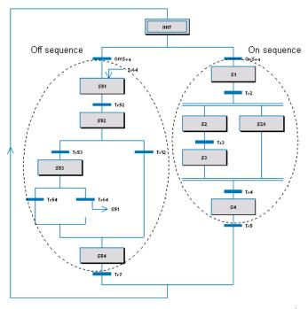
Figure 197. SFC structure configuration example
