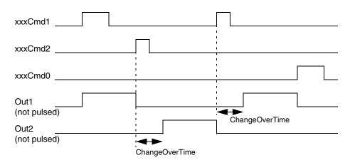
Figure 157. Change-over action state diagram
