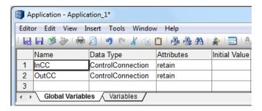
Figure 72. Global variables for connecting the CCTemplate object in the application
