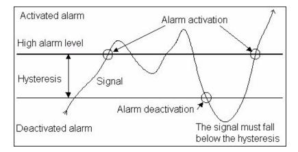
Figure 38. Activation is desired when a signal exceeds a high alarm level
