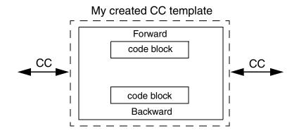
Figure 57. A control module prepared with two code blocks for handling forward and backward directions
