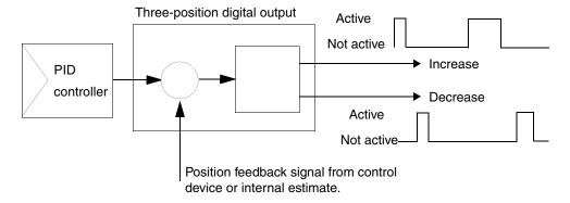
Figure 94. The principle of the three-position digital output function
