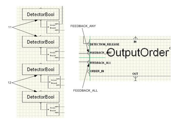
Figure 242. The location of Supply Fire Dampers Closed modules (11) and Extract Fire Dampers Closed modules (12)in the CMD Editor. The OutputOrder module with two feedback connections (depending on action)
