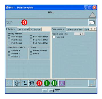
Figure 164. Example of extended faceplate (BiM)
