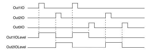
Figure 160. OutputIOLevel state diagram
