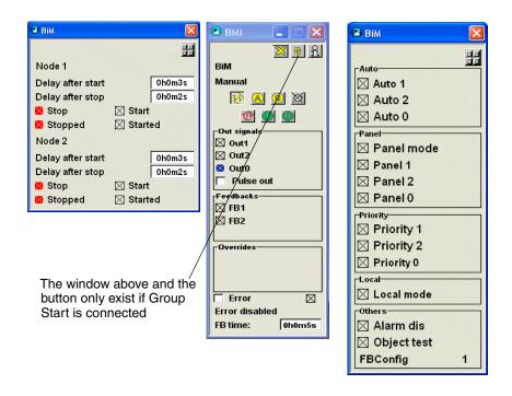
*Figure 165. Control Builder interaction windows for Bi(M)*
