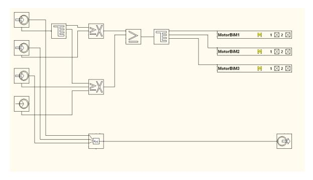
Figure 207. Configuration example of vote logic
