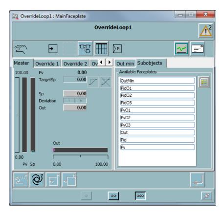
Figure 107. Extended faceplate of OverrideLoop displaying sub objects
