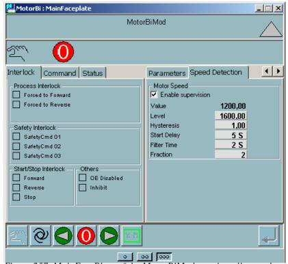
Figure 257. MainFacePlate of the MotorBiMod type in online mode
