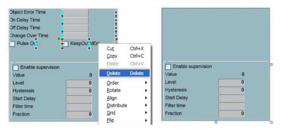
Figure 251. Deletion of a graphics element
