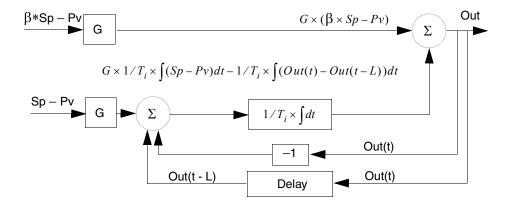
Figure 37. The principle of a PPI controller
