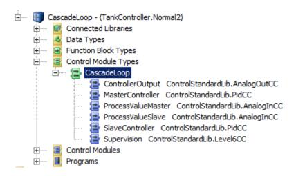
Figure 10. Cascade loop in Control Builder
