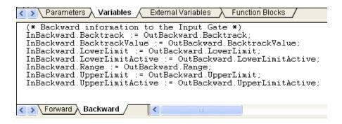
Figure 68. Programming code in the Backward code block
