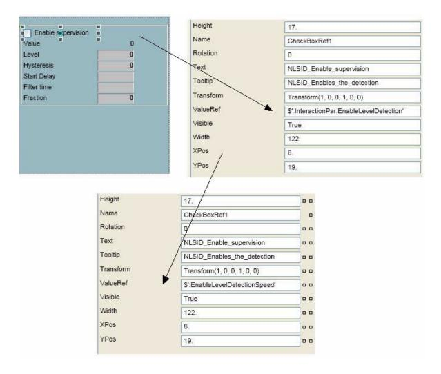
Figure 253. Changing the signals from EnableLevelDetection to EnableLevelDetectionSpeed
