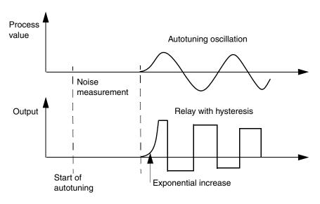
Figure 87. The process value oscillation
