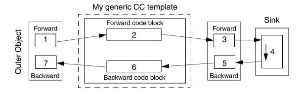
Figure 59. My generic CC template object has a generic solution which simply passes information forward to the next forward object
