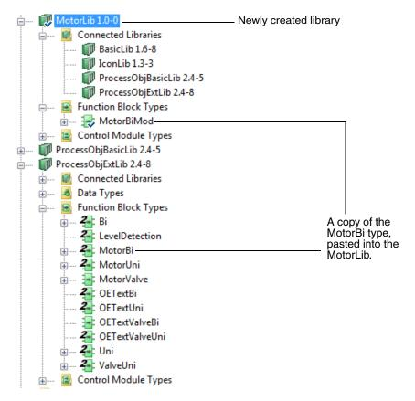
Figure 169. Copying of object types to a new library, MotorLib
