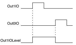
Figure 155. OutputIOLevel state diagram
