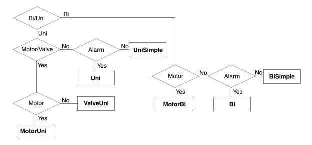
Figure 166. Flowchart of possible process object type choices
