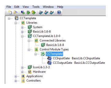
Figure 66. The Gates to ControlConnection are connected to the CCTemplate module
