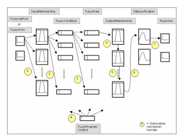
Figure 45. Sub-module connections in the fuzzy controller templates
