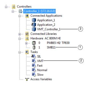
Figure 3. AC 800M High Integrity controller
