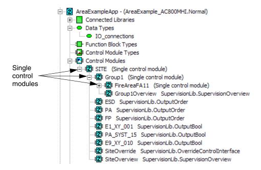
Figure 217. The single control modules represents each level display
