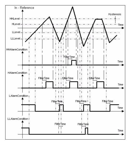
Figure 142. Level Detection example
