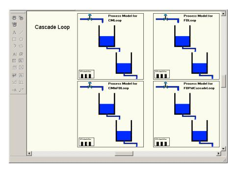
Figure 146. The Cascade Loop application in online mode showing four methods of programming
