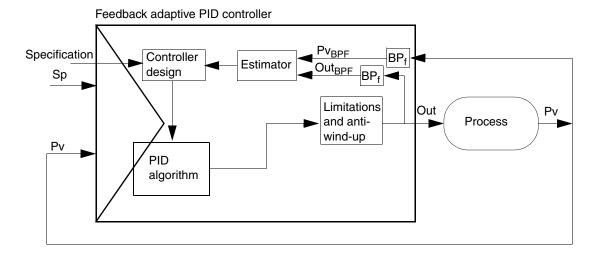
Figure 89. The principle of the feedback adaptive PID controller
