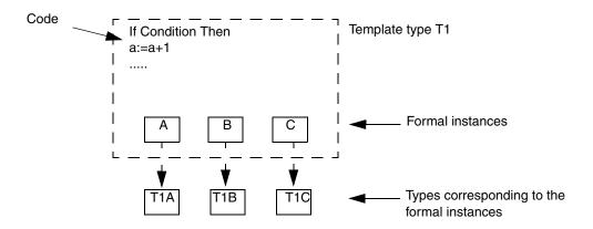
Figure 21. Template type with formal instances
