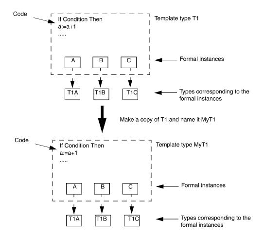
Figure 23. Copying a template type with formal instances
