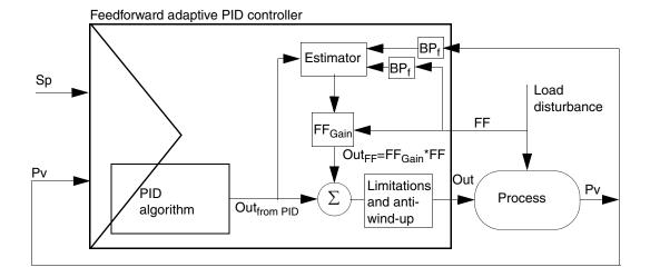
Figure 90. The principle of the feedforward adaptive PID controller
