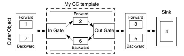
Figure 61. My CC template object is protected by the Gate modules on both sides to ensure a secure signal traffic with ControlConnection
