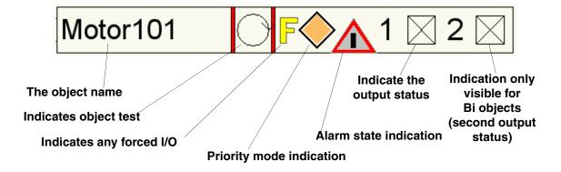
Figure 161. Graphical representation and explanations of the control module icons
