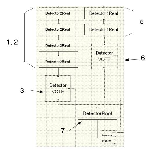
Figure 236. Gas, smoke and MAC configuration, whereas the numbers correspond to the numbered Causes in the fire protection data sheet
