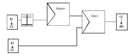
Figure 9. Cascade loop built from control modules
