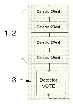
Figure 221. The four Gas detectors and a connected Vote module presented in the CMD Editor in FireAreaFA11
