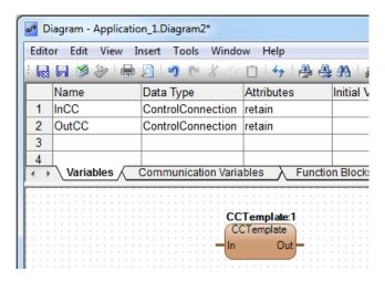
Figure 76. CCTemplate inserted in the graphical code block
