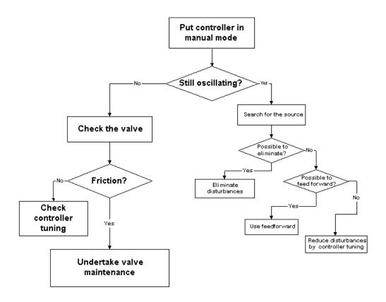
Figure 96. Flow chart for oscillation diagnosis
