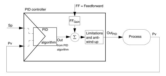
Figure 85. The feedforward principle in the controller
