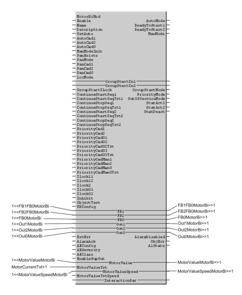
Figure 172. MotorBi function block with connections to variables
