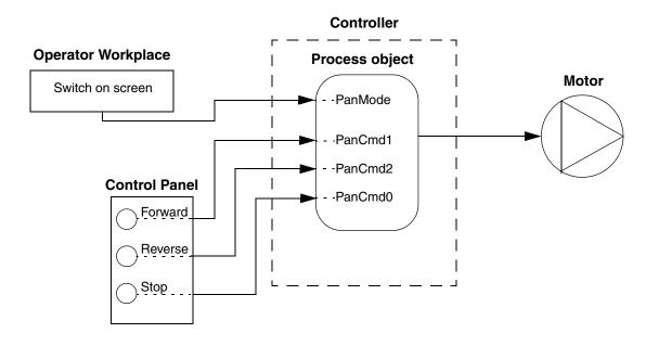
Figure 190. The Panel mode control diagram. A general solution for large applications, where the PanMode parameter is connected to an operator workplace
