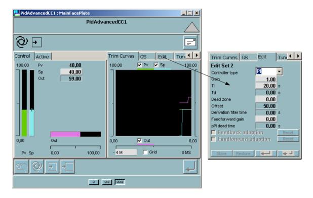
Figure 46. The extended faceplate for the PidAdvancedCC control module with trim curves and parameter settings
