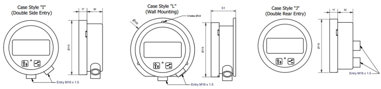
The enclosure must be sealed to at least IP65 rating to ensure correct operation of the electronics Care must be taken when installing assembly to ensure the stated ambient operating conditions are not exceeded. Material Enclosure Stainless steel. Front panel membrane polycarbonate.
