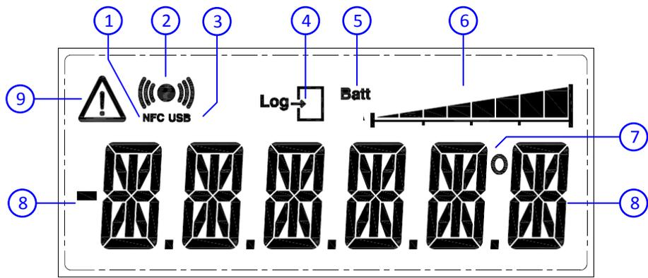
1. NFC - The Symbol is on when a NFC field is detected. When a detected field is lost the symbol will turn off after a few seconds.
