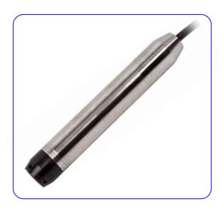
The PTX22 pressure transmitters are high accuracy, robust, 2 wire (4 to 20) mA current output pressure sensing devices used primarily to measure level. They are housed in an all welded stainless steel (316L) assembly containing an oil filled piezoresistive element. Silicon filling and Viton seals are standard with many other options available to order.
