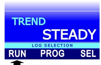
3. The logging of the measurement lines selected for logging is started. The **LOG** indication, the set logging interval and the logging duration appear in the display status bar.
