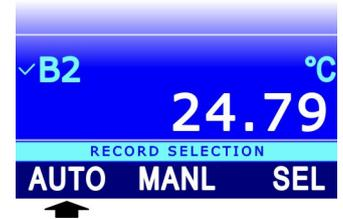
Select the **MANL** command by pressing **F2** to manually acquire a sample.
