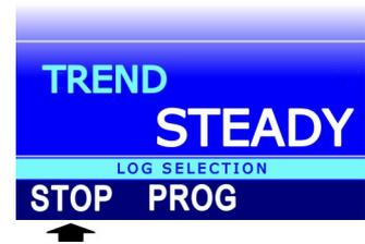
Only the logging start time can be set, in this case it will have to be stopped manually, or only the logging stop time, in this case it will have to be started manually.
