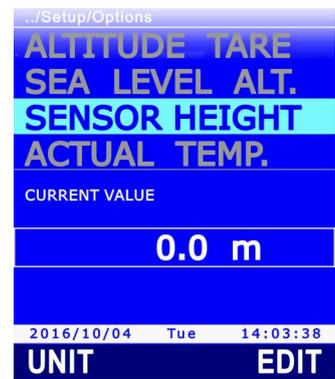
8. For manual setting of the value, select the **EDIT** command by pressing the **F3** key.
