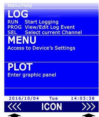
5. To display the help of the symbols appearing in the display status bar, select the **ICON** command by pressing **F2** key.
