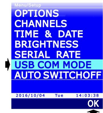
4. Select HID or VIRTUAL COM modes using ▲ and ▼, then press the **F3** key (**OK** command) to confirm.
