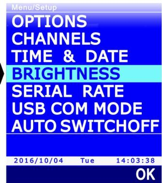
4. Set the brightness level using **▲** and **▼**, then press the **F3** key (**OK** command) to confirm. The available settings are:
