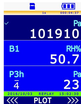
8. Select the <<< (**F1** key) or >>> commands (**F3** key) to scroll the stored data backward and forward in time respectively. To display the graphic trend of the values of one of the stored quantities, select the measurement line using ▲ and ▼, then select the **PLOT** command by pressing the **F2** key (see next paragraph for the details regarding the graph).
