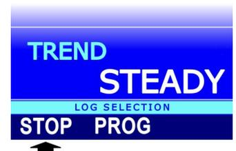
5. After the stop command, the logging stop message appears: wait for the completion of the operation.
