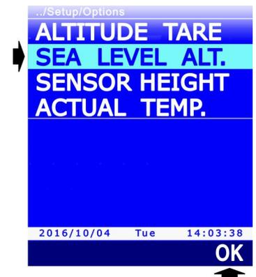
5. The current setting appears. Select the **UNIT** command by pressing the **F1** key to change the measurement unit (m or ft).
