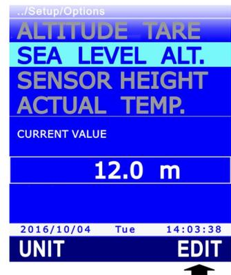
7. Set the first digit using ▲ and ▼, then select the "-->" command (**F2** key) to move to the next digits (the currently selected digit flashes). To return to a previous digit, select the "<--" command (**F1** key). After setting all the digits, press **OK** (**F3** key) to confirm the value.
