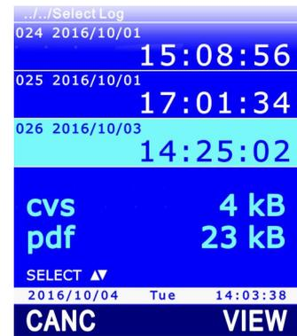
7. To access the data recorded in the selected logging session, select the **VIEW** command by pressing the **F3** key. The stored data appear on the display. The green line under the measurement area shows the date and the time of the displayed sample. The orange line over the measurement area shows:
