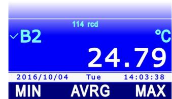
4. The indication of the performed selection is shown in the upper part of the measurement line, next to the number of the acquired samples.
