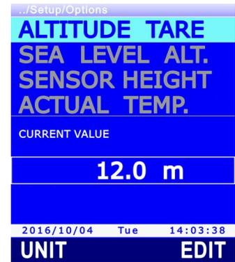
8. For manual setting of the reference value, select the **EDIT** command by pressing the **F3** key.
