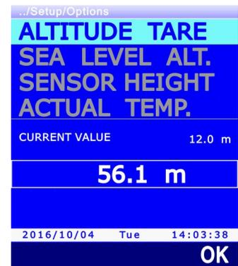
Selecting the **MANUAL ENTRY** option, the current setting of the reference value appears. Select the **UNIT** command by pressing the **F1** key to change the measurement unit (m or ft).
