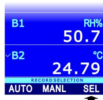
4. The indication "0 rcd" appears on the upper part of the measurement line, to indicate that the quantity has been selected for the RECORD function.
