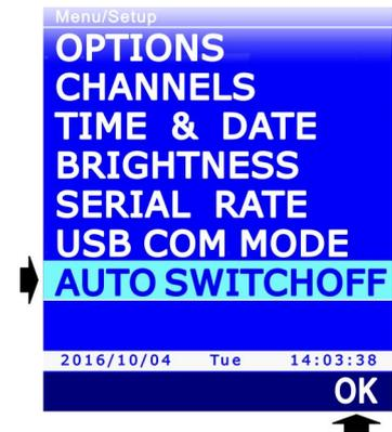
4. Set the number of minutes using ▲ and ▼, then press the **F3** key (**OK** command) to confirm.
