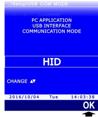
5. The instrument returns to the USB COM MODE item, press **ESC** twice to exit the menu.
