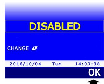
5. The instrument returns to the **AUTO SWITCHOFF** menu item, press **ESC** twice to exit the menu and return to the measurement mode.
