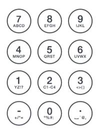
The alpha-numeric keys are used for entering text and values with the operator panel. When pressing shortly, the numeric value (0 - 9), minus sign (-), or decimal point / dot (.), is selected.
