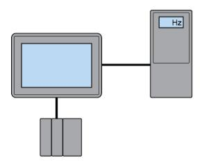
*Figure 27. The operator panel communicating with one controller and one frequency converter.*
