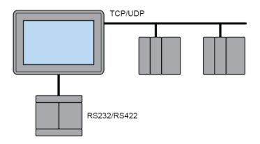
*Figure 28. The operator panel communicating in series with one controller via Ethernet and with controllers of another make.*
