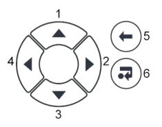
The navigation keys are used for moving the cursor between objects, and for editing text and values.
