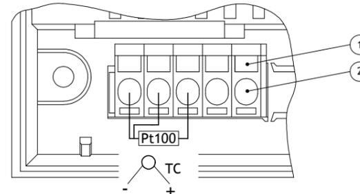
To make a connection: Insert small screwdriver blade into tension clamp orifice, (1) push and twist to deflect clamp into open position. Do not lever screwdriver thus forcing connector body sideways. Insert conductor tail sufficiently into (2) then release screwdriver. Ensure no loose wire strands protrude.
