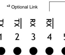
\*2 Connection of the link connects a 100 ohm termination resistor across pins 4 and 5. This resistor should only be selected for the instrument furthest away from the host. Full details of the modbus protocol are supplied separately with the pod.
