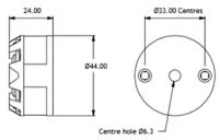
Mounting holes: two holes 4.8 mm diameter, 33 mm centres.
