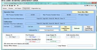
The diagnostic log tab can be set to record a log onto the SEM210. A 150 point rolling log set at time intervals between 5 s up to 1 hr can be recorded for viewing or can be saved to a text file.
