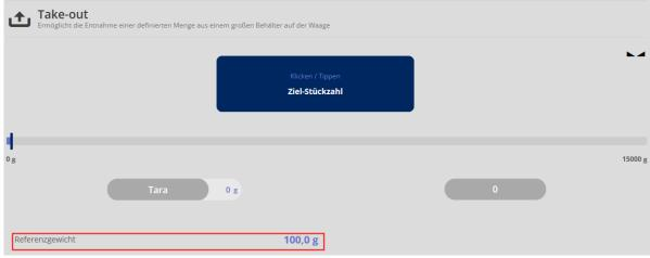
Click the blue field "Target piece quantity". Enter now the target piece quantity (=piece quantity of the removed parts) and enter the target tolerance: **Here is an example:**
