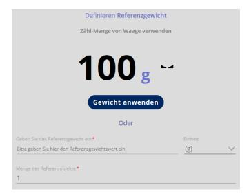
Click button "Apply weight", and then click "Confirm". The screen for entering the target piece quantity appears. The reference weight is shown below:
