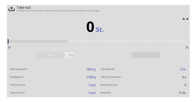
Now remove the pieces until the target weight is reached. The green bar graph shows this, also an acoustic signal sounds when the target weight is reached.
