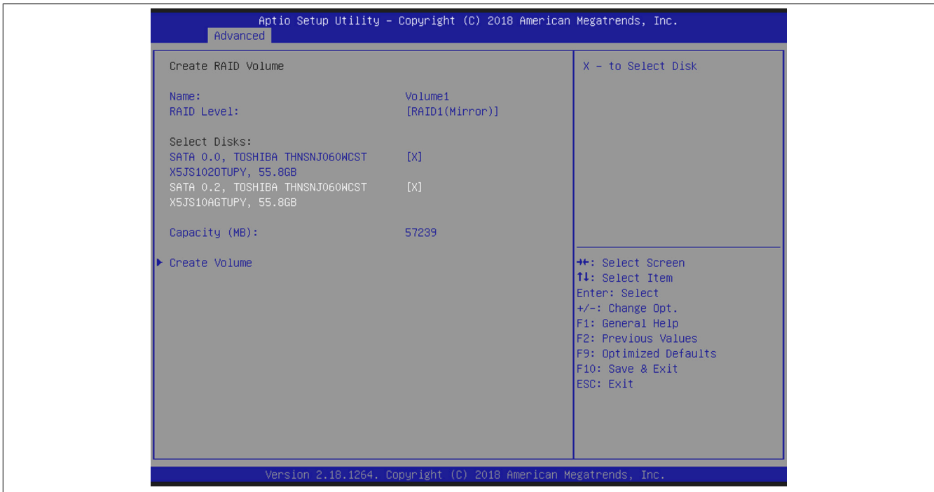
Figure 32: Configuration of the new RAID volume
