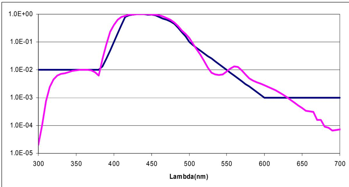
Figure 9: comparison between spectral response curve obtained by the combination of channels (in purple color) and weighting curve  $B(\lambda)$  (in black)
