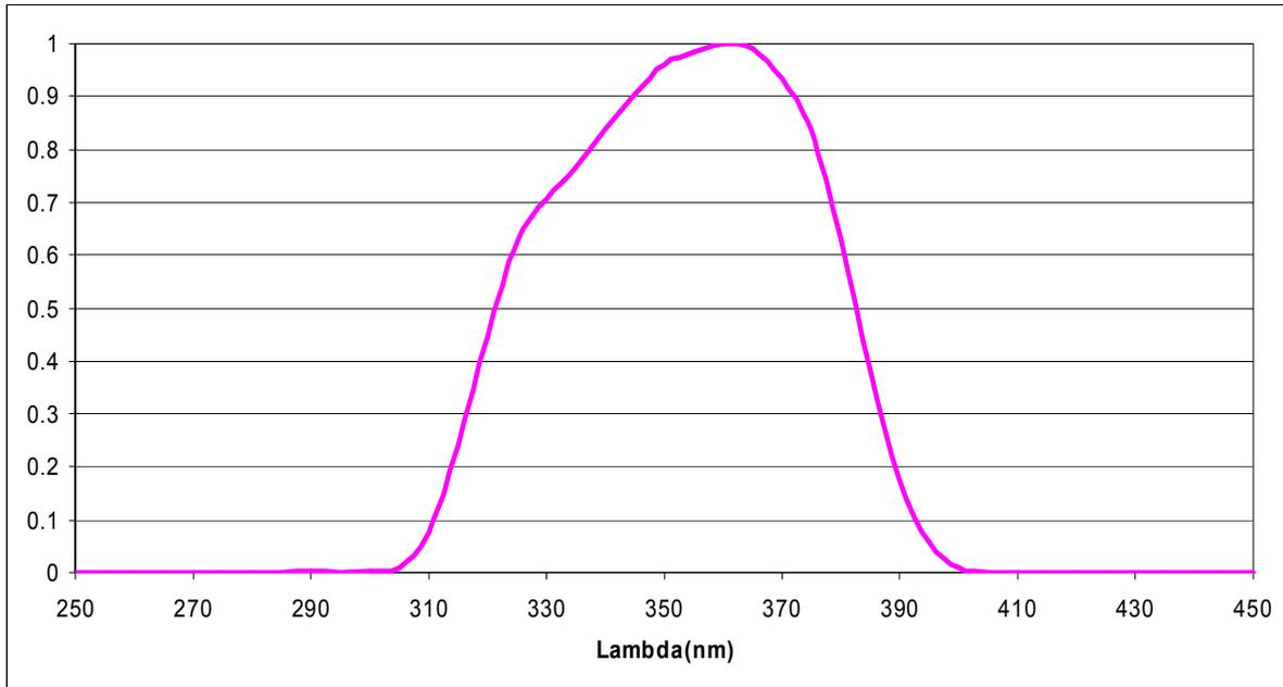
Figure 8: spectral response curve of UVA sensor
