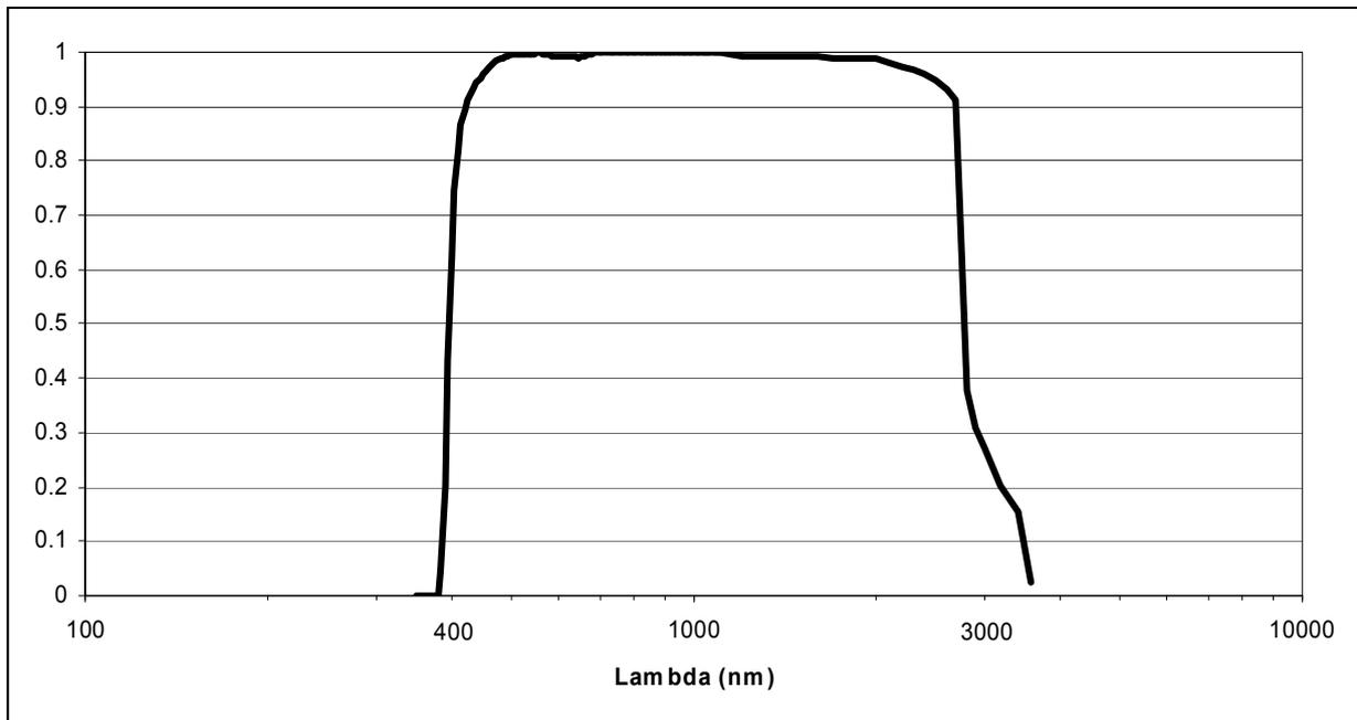
**Figure 12: spectral response curve of the pyranometer.**
