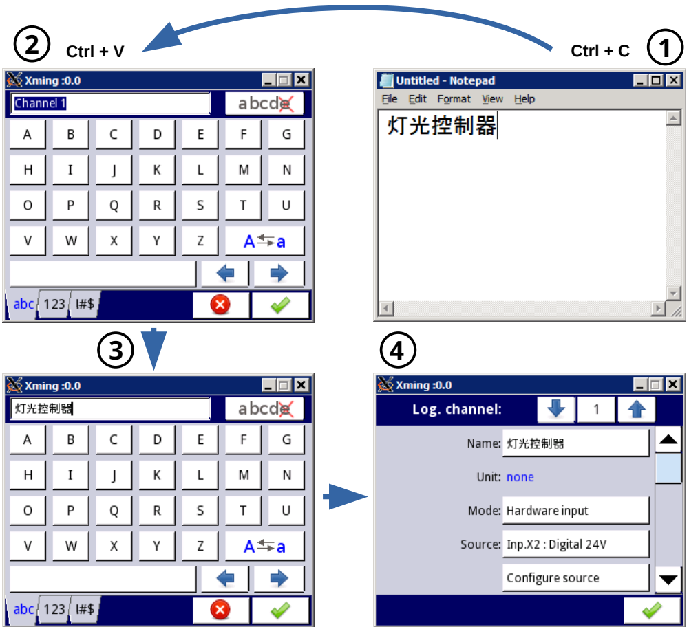
Fig. 7.15. The flowchart for entering characters that are not available from the device menu
