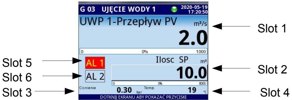
Fig. 7.160. Slots layout in controllers view
