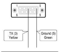
Use the delivered cable to connect the remote display to the weighing transmitter. It is not allowed to extend the cable to a length more than 50m.
