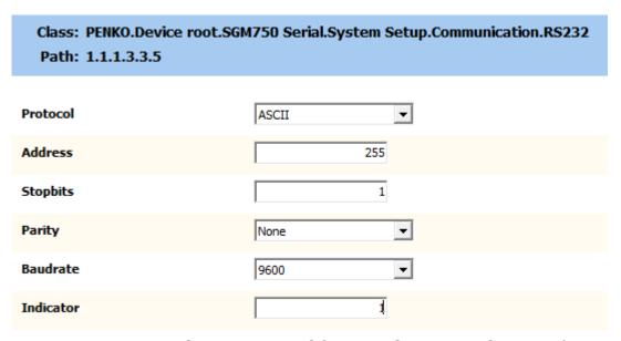
Make sure that only RS232 is set to ASCII, the RS232 and RS422 can't be both set to ASCII at the same time.
