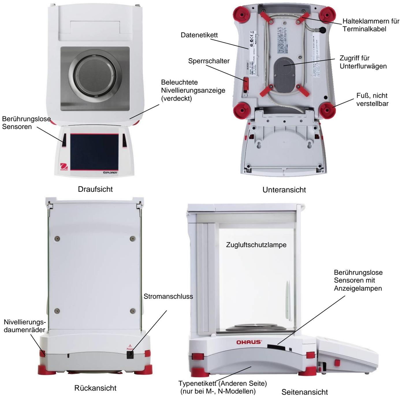
Abbildung 3-2. Explorer-Waage (Modelle EX124, EX224, EX324, EX223, EX423, EX623, EX1103)
