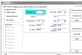
The **S-Toolkit** enables reading and writing operations of configuration, updating the device firmware and obtaining basic information through RS-485 serial interface. This application enables to quickly and easily define device parameters in one of three possible configuration models. The set of parameters can be transmitted directly to the device or stored in a file for future use.
