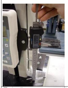
Move the slider up until the distance is > 60mm. Don't care about the exact distance, you can input the caliper reading into the software to fix the calibration
