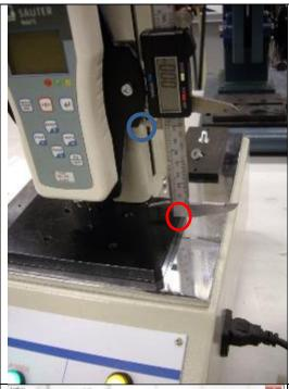
Move the slider to the down until the limit switch stops the movement. Take a caliper and measure the distance between the base plate (red marked) and the ground plate (blue marked) from the FL. If possible zero the caliper.
