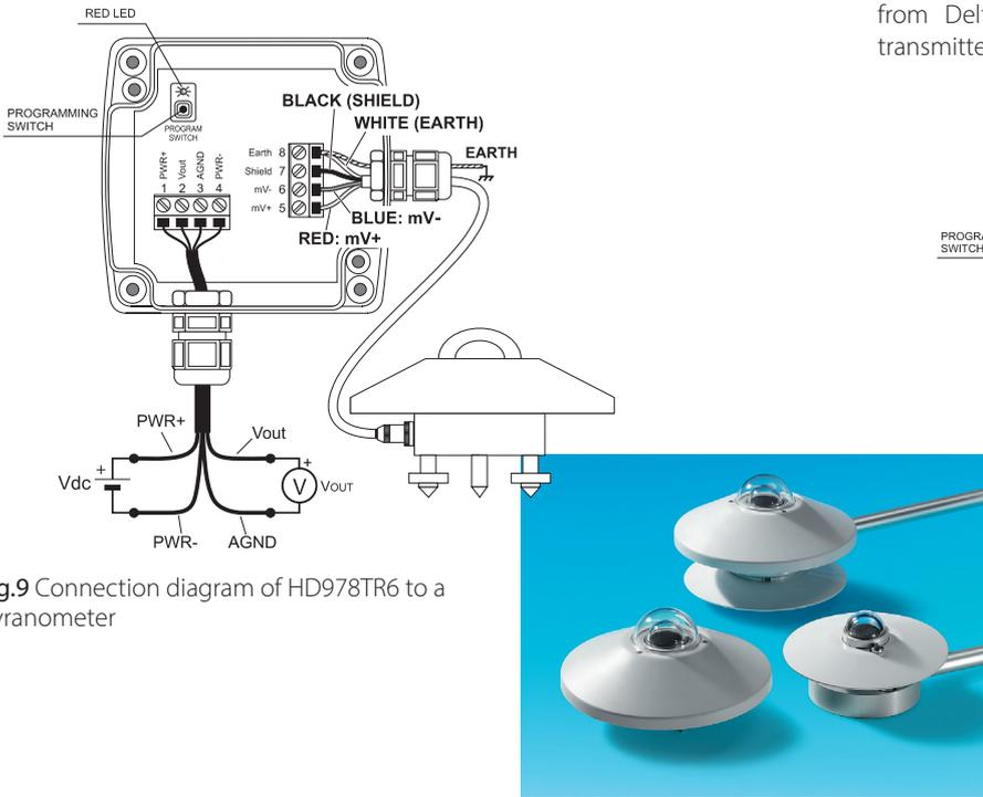
Fig.9 Connection diagram of HD978TR6 to a pyranometer
