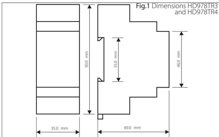
The instrument is housed in a 2 modules DIN (Width 35mm) container with standard connection for 35 mm rail for the models HD978TR3 and HD978TR4; a wall mount container for the models HD978TR5 and HD978TR6.
