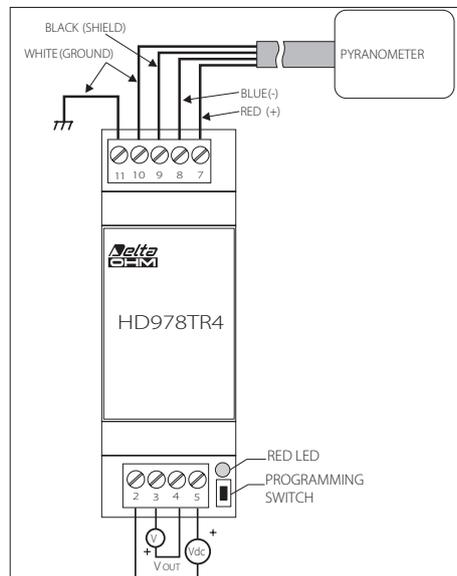
Fig.6 Connection diagram of HD978TR4 to a pyranometer
