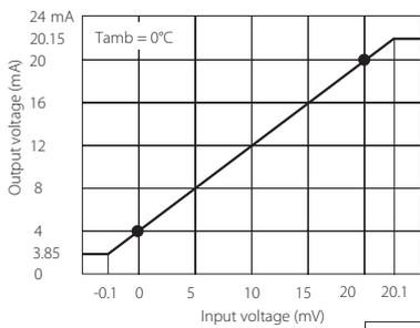
Fig. 3 HD978TR3 and HD978TR5 continuous current measure
