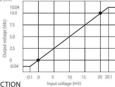
Fig. 4 HD978TR4 and HD978TR6 continuous voltage measure
