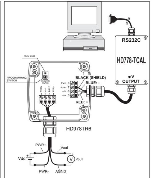
Fig. 13 Connection diagram for programming HD978TR6 with HD778-TCAL
