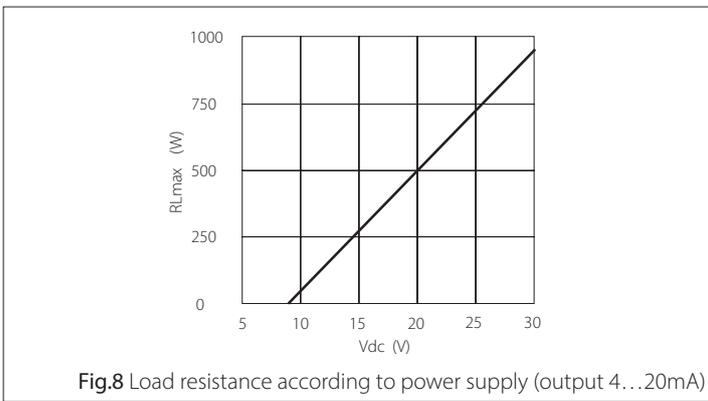
Fig.8 Load resistance according to power supply (output 4...20mA)
