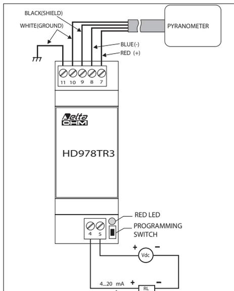
Fig.5 Connection diagram of HD978TR3 to a pyranometer.
