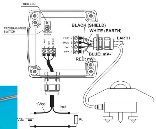
Fig. 10 Connection diagram of HD978TR5 to a pyranometer
