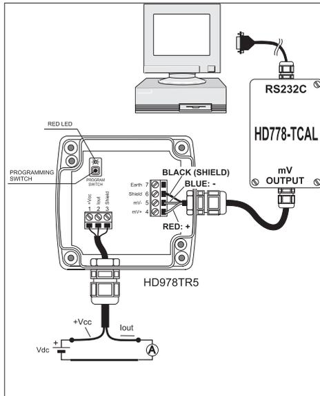
Fig. 12 Connection diagram for programming HD978TR5 with HD778-TCAL
